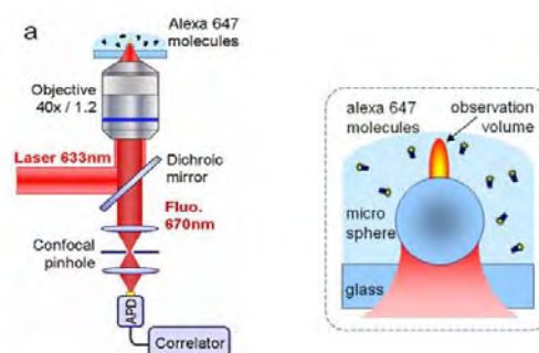
Fig. 1: Left panel: Sketch of the experimental configuration. Right panel: close-up on the microsphere.
