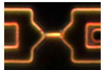
Fig. 4: Single silicon nanowire trapped between electrodes
